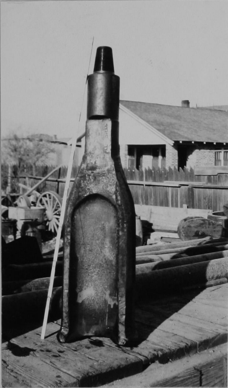
Fig. 10.- The type of bit ordinarily used in water well work.
