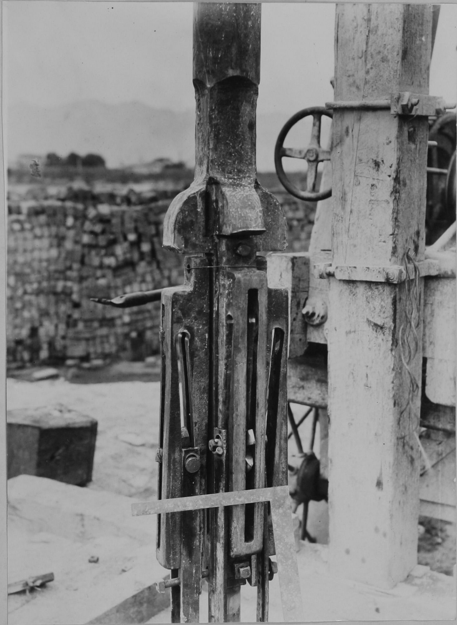
Fig. 21.-The Star Four-Way Perforator only partly assembled but showing how the rolling knives work in the grooved slots.
