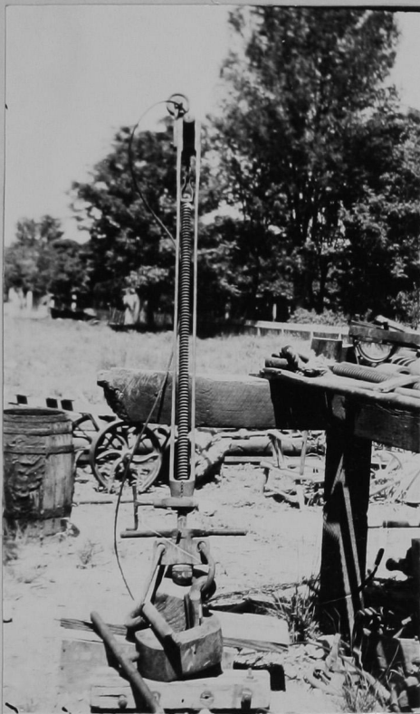
Fig. 14.- Temper screw; note the heavy construction of the cable clamps.
