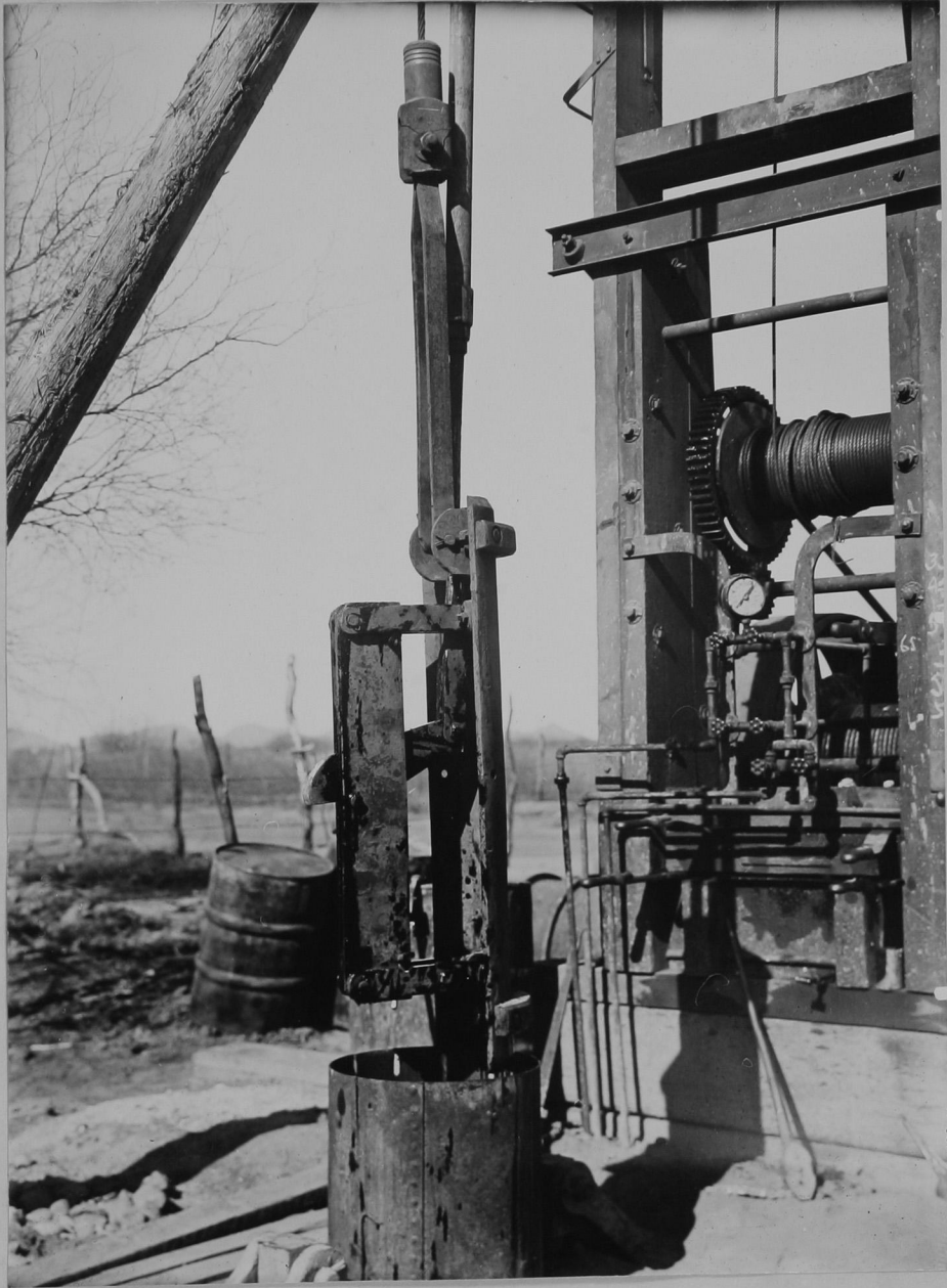
Fig. 20.- A 16-inch Mills Knife Perforator backed up to use in 18-inch casing.
