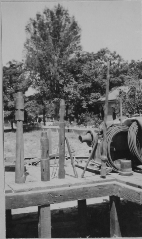
Fig. 12.- A group of fishing tools looking from left to right consisting of horn socket, combination socket, slip socket, and slips, rope knife and rope spear.
