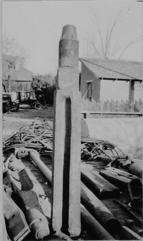
Fig. 11.- A Mother Hubbard or all steel hard rock drilling bit.
