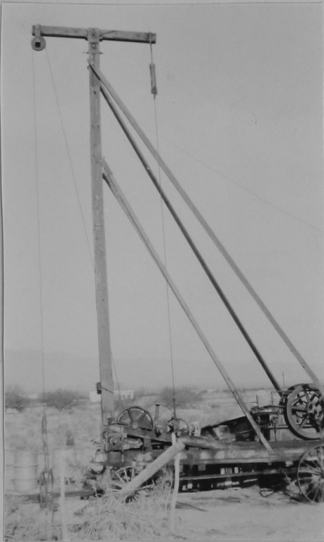
Fig.4.- A small California type rig which is not equipped with a sand line or hydraulic pump.
