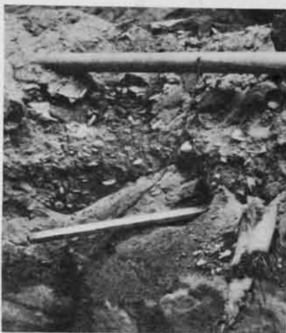
Fig. 2—Finding of a sawed plank on rock bench at top of inner gorge, buried deep in undisturbed river fill, gave conclusive proof of great depth of scour in recent times.
